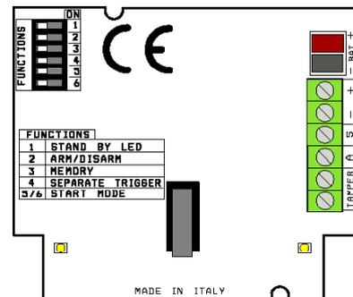
**TAMPER:** N.C. Antiopening and Tearing Off Contact
